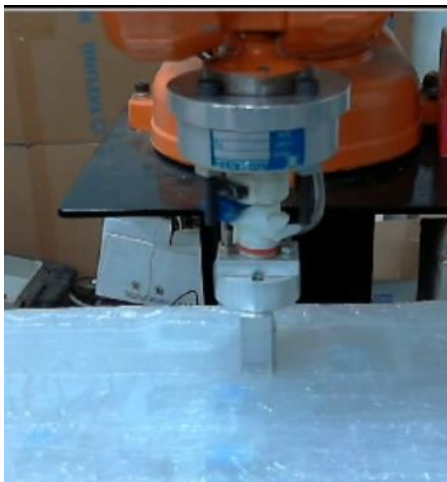
Fig. 6 The ABB Robot Equipped with Force Sensor and Palpation Probe
