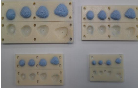
Fig. 5 The Fabricated Tumor Phantom Modules
