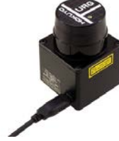
Figure 3 Laser range finder (URG-04LX-UR01) used for obstacle detection.
