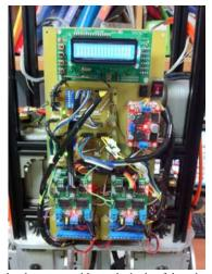
Fig. 13. Electric hardware assembly on the body of the robot.
