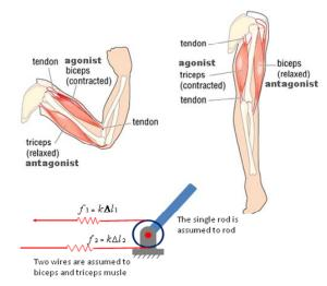
Fig. 1. Illustration of biomechanics arm movement of a BTDJ module.
