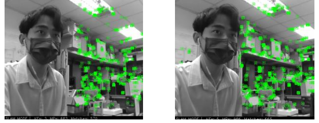
Fig. 5 Comparison of the results : (a) ORB-SLAM2 and (b) the proposed method.
