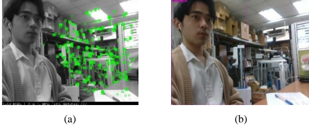
Fig. 3 (a) Result after feature points reprojection and (b) The detection bounding box.
