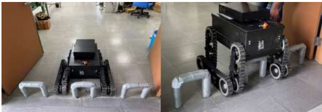
Fig. 9. The elevated mode enables the robot to elevate its body, allowing it to directly overcome obstacles without the need for detours.
