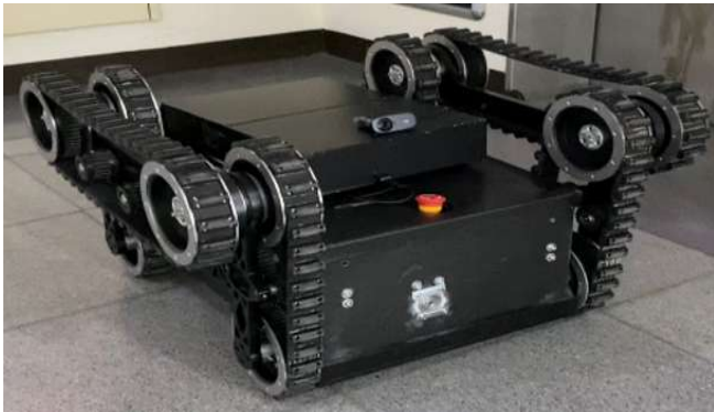
Fig. 8. The four-wheel mode reduces the contact area, allowing the transformable tracked robot to increase speed and reduce energy consumption on flat surfaces.
