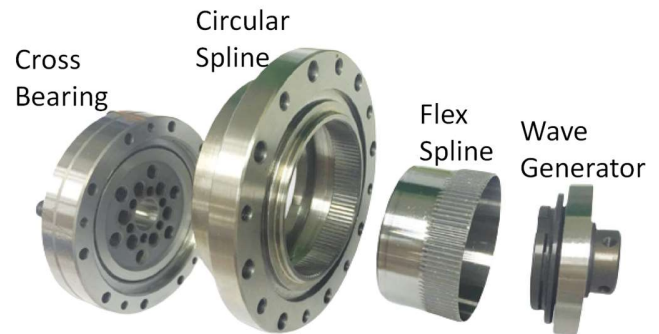
Fig. 1 The HD reducer used for accelerated life testing.
