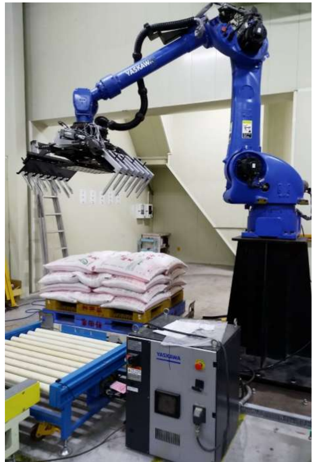
Figure 4. Depicts the application of the gripper mechanism developed in this research on the YASKAWA robot.
