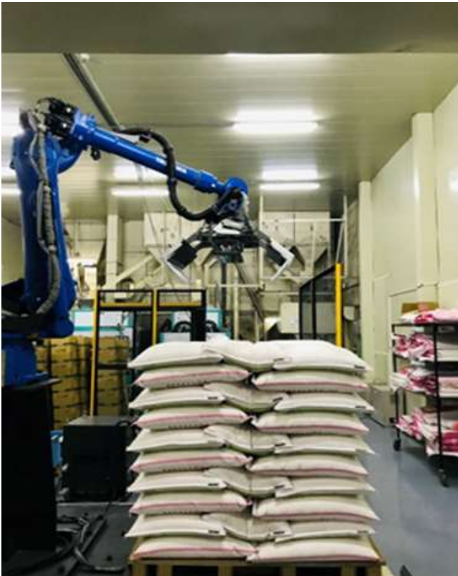
Figure 13. Factory floor image of rice stack after completing the palletization using proposed system.
