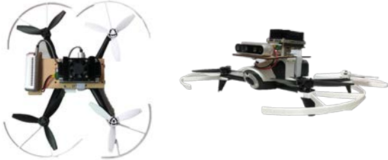
Figure 3. Physical picture of the experimental autonomous quadrotor: (a) top view of the complete experimental set-up; (b) exploded illustration of NVIDIA Jetson TX2 and Intel RealSense depth camera.
