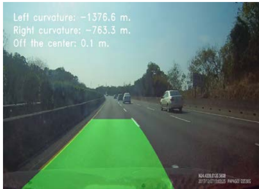
Fig. 6. Transformation to the original perspective and calculation of lane curvature and lane offset.
