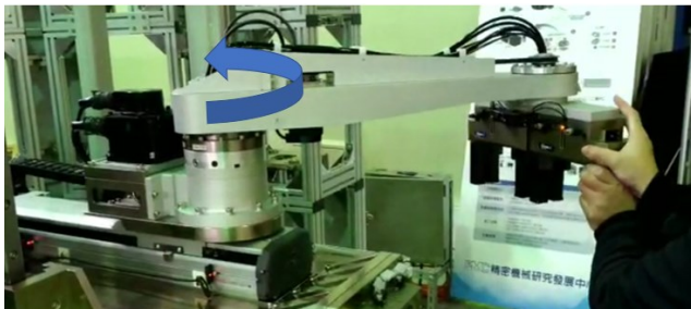
Fig. 7. Manual Teaching Mode for the 2 nd joint.
