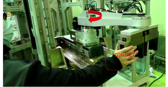
Fig. 11. Collision test on 2 nd joint.
