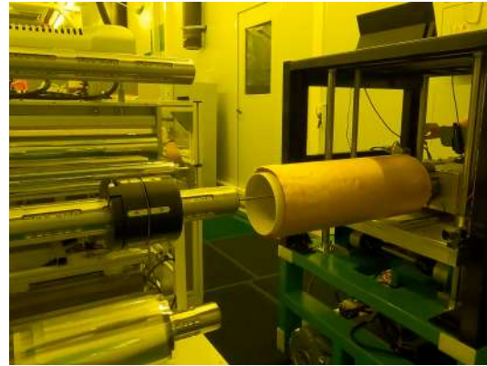
Fig. 26. OAMR loading operation
