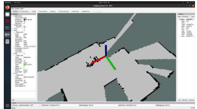
Fig. 20 Comprehensive map of layout using SLAM
