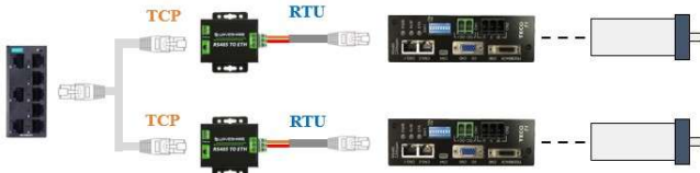
Fig. 16. Gripper positioning control architecture
