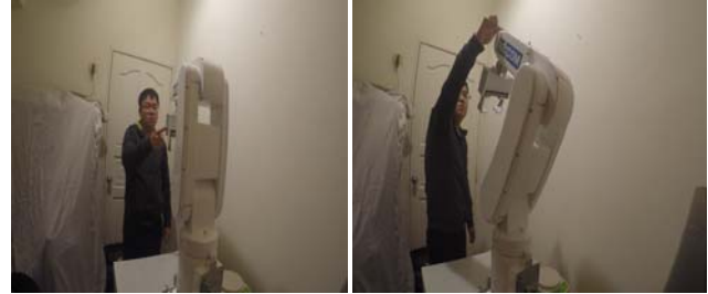
Figure 10. Two still pictures of the HIWIN manipulator moved by using only one finger when only both friction compensation and gravity compensation methods are used.
