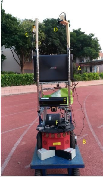
Figure 3. The equipment used in the experiments. It includes a laptop computer, a mobile platform, a GPS receiver, an IMU, an RGB-D camera, and an external power source.
