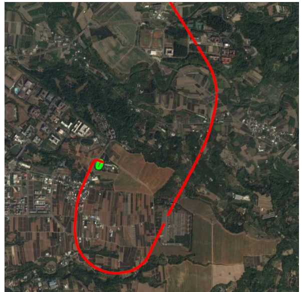
Figure 7. The trajectory from EKF with IMU. The result shows that IMU is not able to provide a reasonable trajectory.
