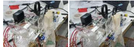
Part 2: The V-shaped constraints fix bag in place, and then the C-shaped jaws tighten bag opening
