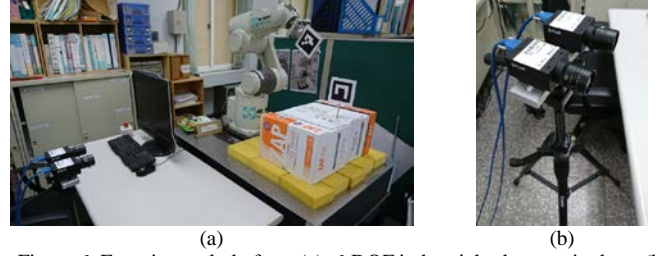
Figure 6. Experimental platform (a). 6-DOF industrial robot manipulator (b). stereo camera.
