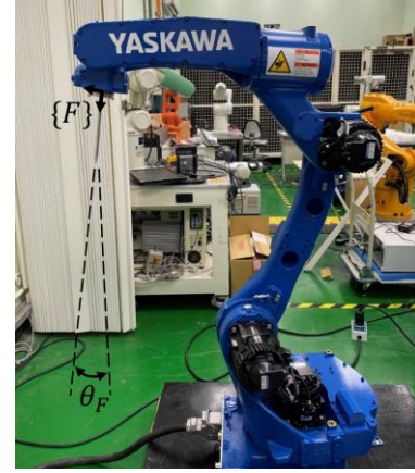
Fig. 13. Experiment of the planar translation calibration by varying the flange inclinations \theta_F
