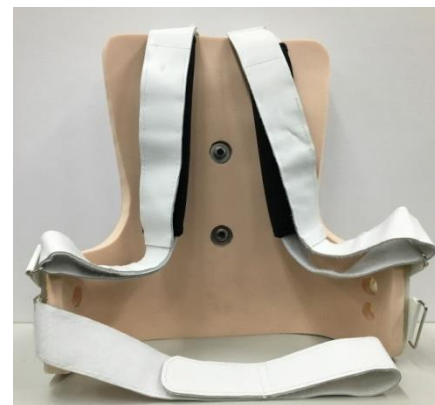
Figure 3. The backpack for holding HAMEXO.
