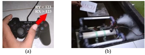
Fig11. (a) Joystick Command Movement Forward (b) ROV Movement Forward
