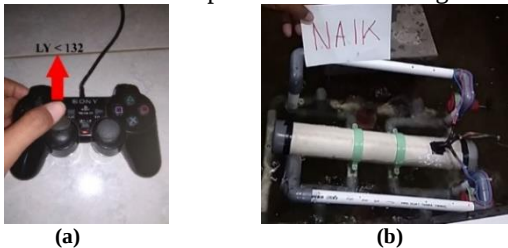
Fig 9 (a) Joystick Command Movement Up (b) ROV Movement Up
