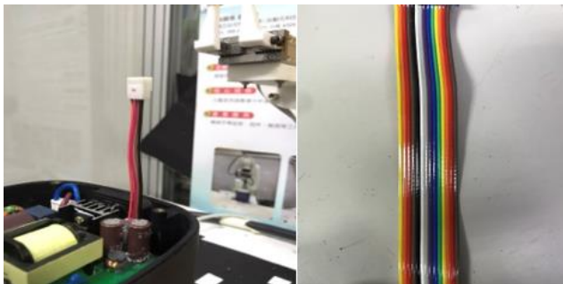
Fig. 14. Color of connector wire hindering insertion
