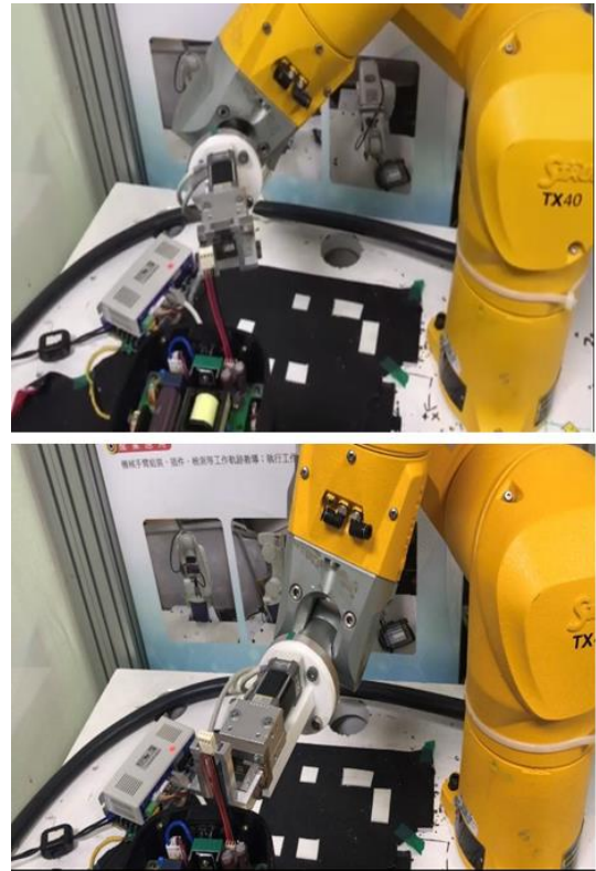
Fig. 11. Limit on rotation angle of connector around Z-axis: 25 degrees (up) and -25 degrees (down)
