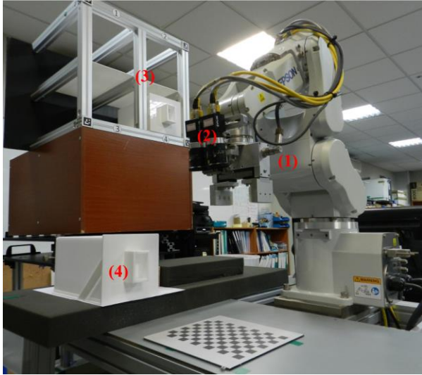
Fig. 1. The warehouse automation system. (1) Robot arm, (2) stereo camera c , (3) frame f (store magazines), and (4) magazine.
