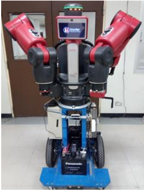
Fig. 1. The mobile manipulator system developed for fetch-and-carry tasks
