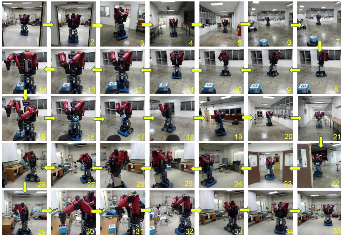
Fig. 20. Fetch-and-carry operation sequence of the robot
