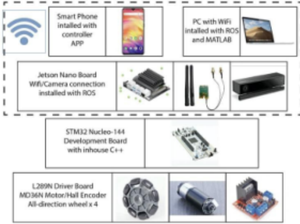
Figure 1. Omni-vehicle system architecture. The whole system has three structure: top/mid/bottom. Where the top consists of mapping and remote-control via WiFi. The mid structure joins the top/bottom for the vehicle's movement and location recording.
