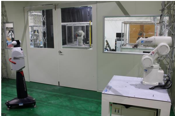
Figure 7. experiment setup: robot and laser tracker.
